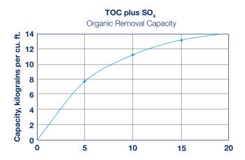
Capacity based on 2 gpm/cu.ft. flow rate, pH near neutral, and 36 inch minimum bed depth. Capacity is for TOC plus sulfate. No engineering downgrade has been applied.
