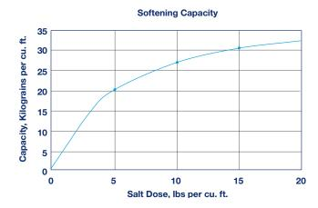
Capacity and leakage data are based on the following: 2:1 Ca:Mg ratio, 500 ppm TDS as CaCO<sub>3</sub>, 0.2% hardness in the salt and 10% brine concentration applied co-currently through the resin over 30 minutes. No engineering downgrade has been applied.
